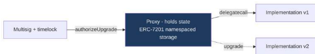
Figure 10 — UUPS upgrade flow with namespaced storage.
